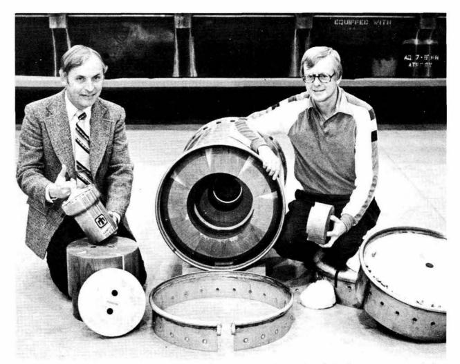
PATENT AWARDED—Inventors Ken Cole (5656) and John Andersen (1721) display components of their plutonium shipping container. The cask, weighing some 500 lbs., survived a severe testing program without leaking. It will be used to ship up to 4.4 lbs. of solid plutonium between nuclear reprocessing plants, storage sites, fabrication plants and research facilities.
